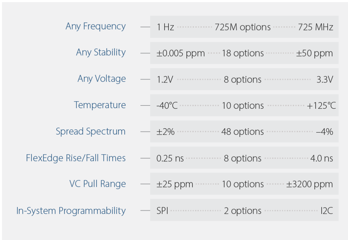
Figure 7: Unlike quartz XO, SiTime MEMS XOs offer a wide range of configuration options, to enable designers to meet exact application requirements
