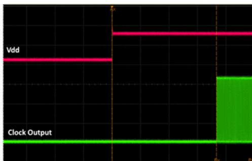
Figure 17. Startup Waveform vs. Vdd
