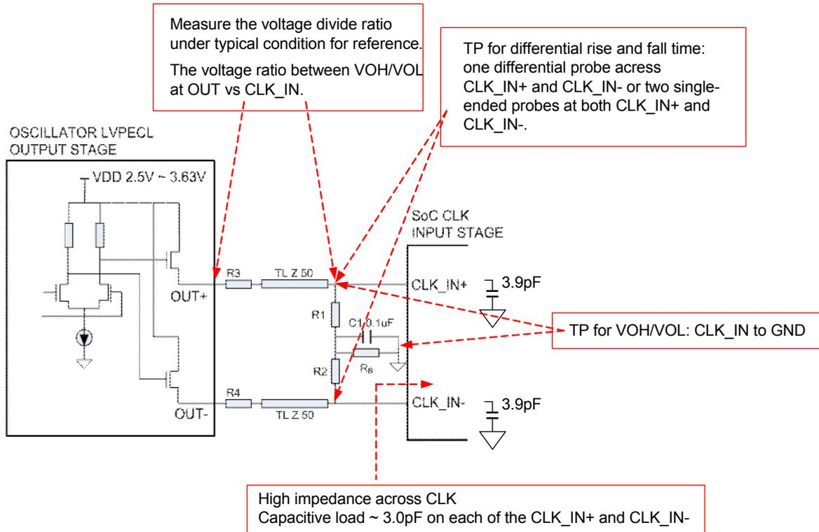
\* Customize termination circuit uses  $R1=R2=R3=R4=R6=51$  ohms with operating VDD from 2.5V to 3.63V.
