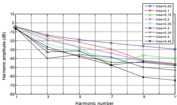
**Figure 2. Harmonic EMI reduction as a Function of Slower Rise/Fall Time**
