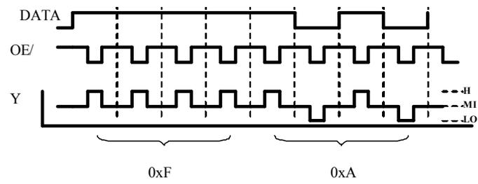
**Figure 8. Signal Polarity**
