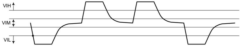
**Figure 7. Tri-State Signal Generated with Tri-State Buffer**
