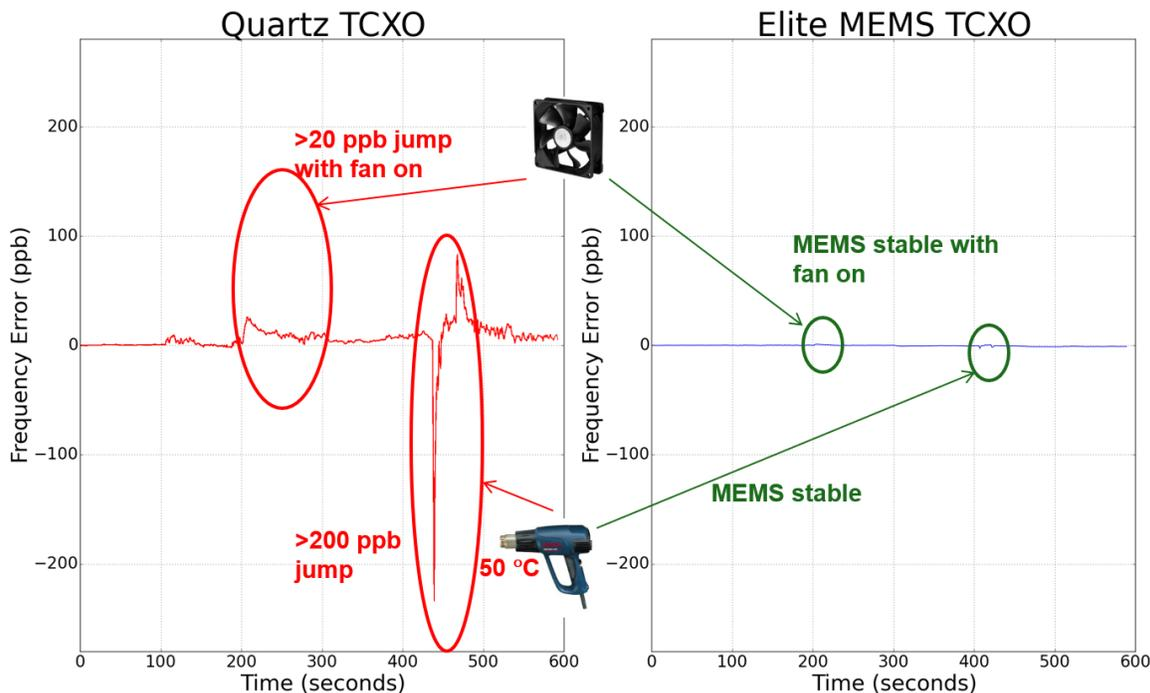
Figure 2. Quartz TCXOs are sensitive to heat, airflow, and rapid temperature shifts, exhibiting significant frequency variations, while MEMS TCXOs are extremely stable under these conditions.
