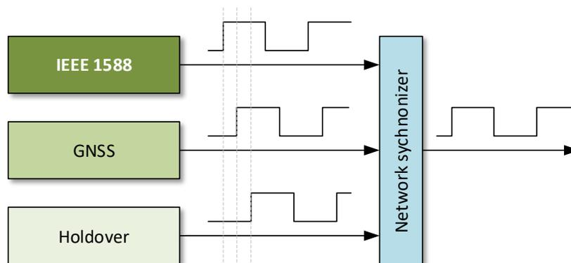
Figure 1. One of three timing sources is selected by the network synchronizer, with no phase jumps during switching.
