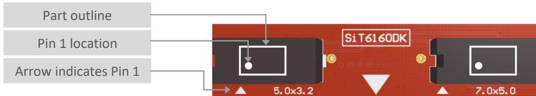
**Figure 8. Time Machine socket card SiT6160DK.**
