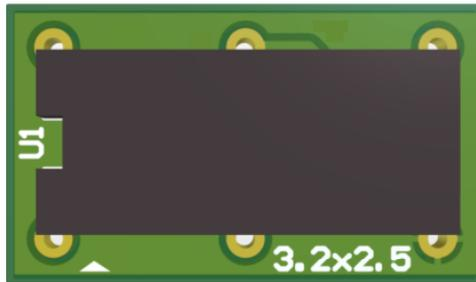
**Figure 5. Time Machine interposer board SiT6142IB.
