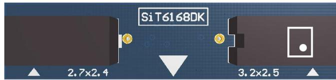
**Figure 12. Time Machine socket card SiT6168DK.
