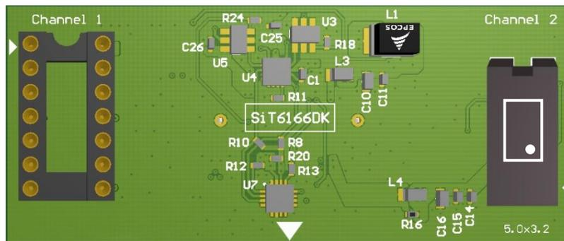
**Figure 13. Time Machine socket card SiT6166DK.
