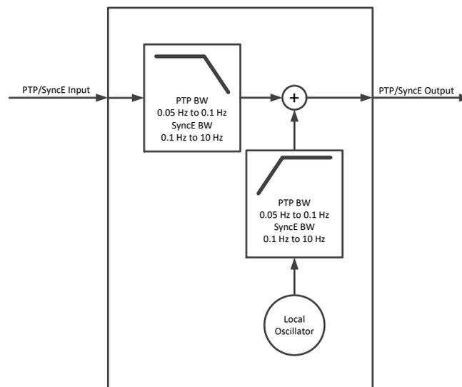
Figure 1: PTP system node simulation model
