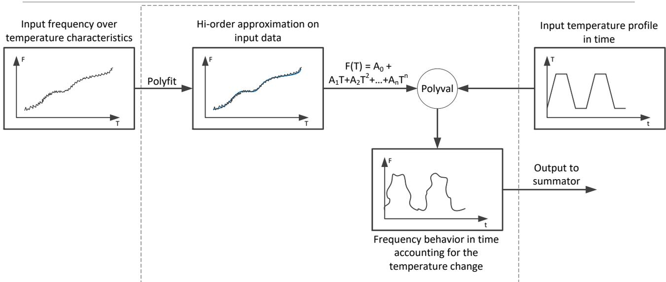
Figure 6: Variable temperature effect simulation model
