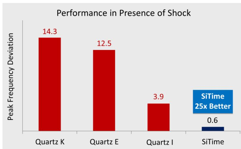
Figure 2: Oscillator sensitivity to 500-g shock
