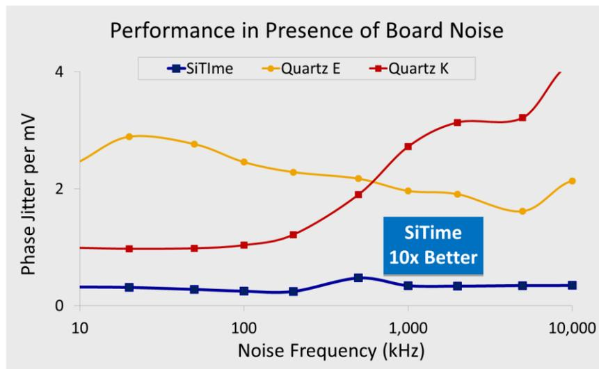
Figure 4: Phase jitter in the presence of 50 mV peak-to-peak power supply noise for SiTime MEMS oscillator (lower line) and quartz oscillators as a function of power supply switching noise frequency
