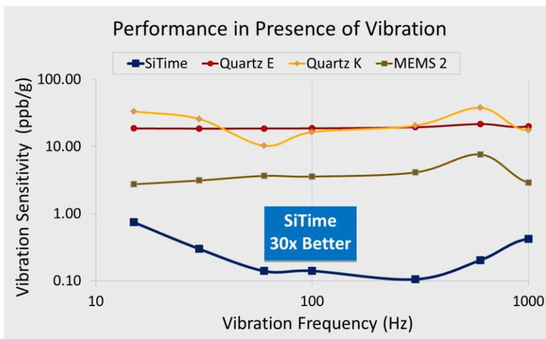
Figure 1: Oscillator sensitivity to sinusoidal vibration
