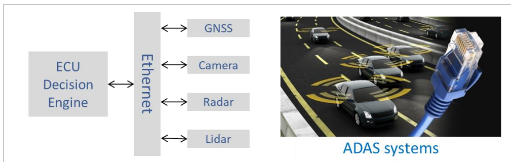
Figure 4: Low-jitter MEMS oscillators are resistant to shock, vibration, power supply noise, and thermal gradients, making them ideal for clocking Ethernet, PCI-Express, and SerDes/PHY in ADAS systems
