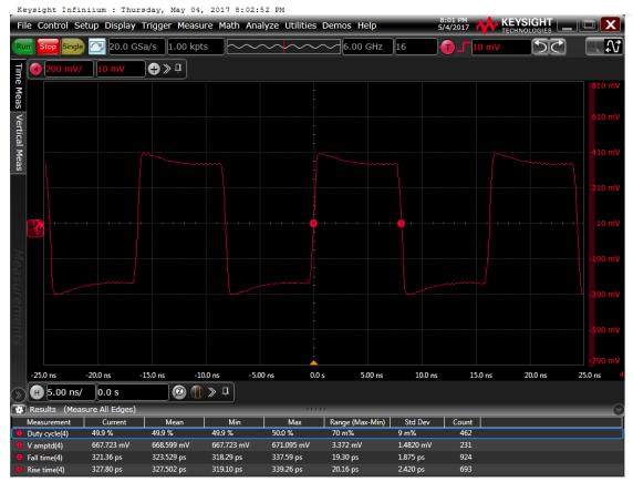
Figure 6: Output waveform, 2.5 V
