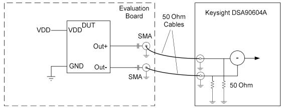
Figure 2: Test setup for measuring period jitter
