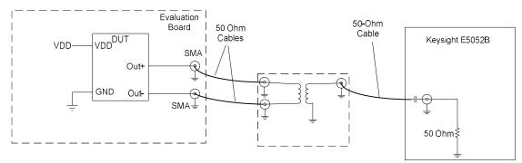
Figure 3: Test setup for measuring phase noise.
