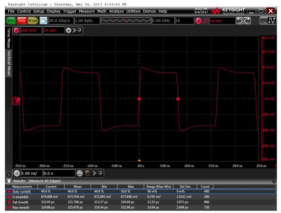
Figure 7: Output waveform, 3.3 V
