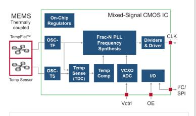
Patented architecture with DualMEMS, noiseless temperature sensing and TurboCompensation
