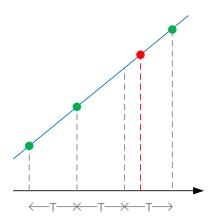
When an ADC is used, jitter causes quantization errors. When excessive jitter is present on a clock, in other words when a clock edge comes too early or too late, an ADC samples the incoming signal at the wrong moment. Incorrect values in the data stream can significantly hamper the functionality of a system.
