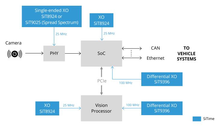
A camera, either infrared or visible wavelength, monitors the driver's face. Data is sent to an image processing system based on an SoC and a machine-learning vision processor, which can be either internal to the SoC or external as shown here. In the latter case, data transfer between the two is usually done via a PCI-Express interface, which offers both the required low latency and high bandwidth.
