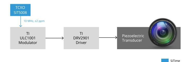
The TI ultrasonic lens cleaning system requires a single 10 MHz oscillator as a clock source with a recommended ±5 ppm stability over temperature. The MEMS-based SiT5008 TCXO meets this requirement in a very small footprint (2.5 x 2.0 mm). If ultra low power and a smaller form footprint (1.6 x 1.2 mm) is desired, the ±25 ppm SiT1623 oscillator can be used.
