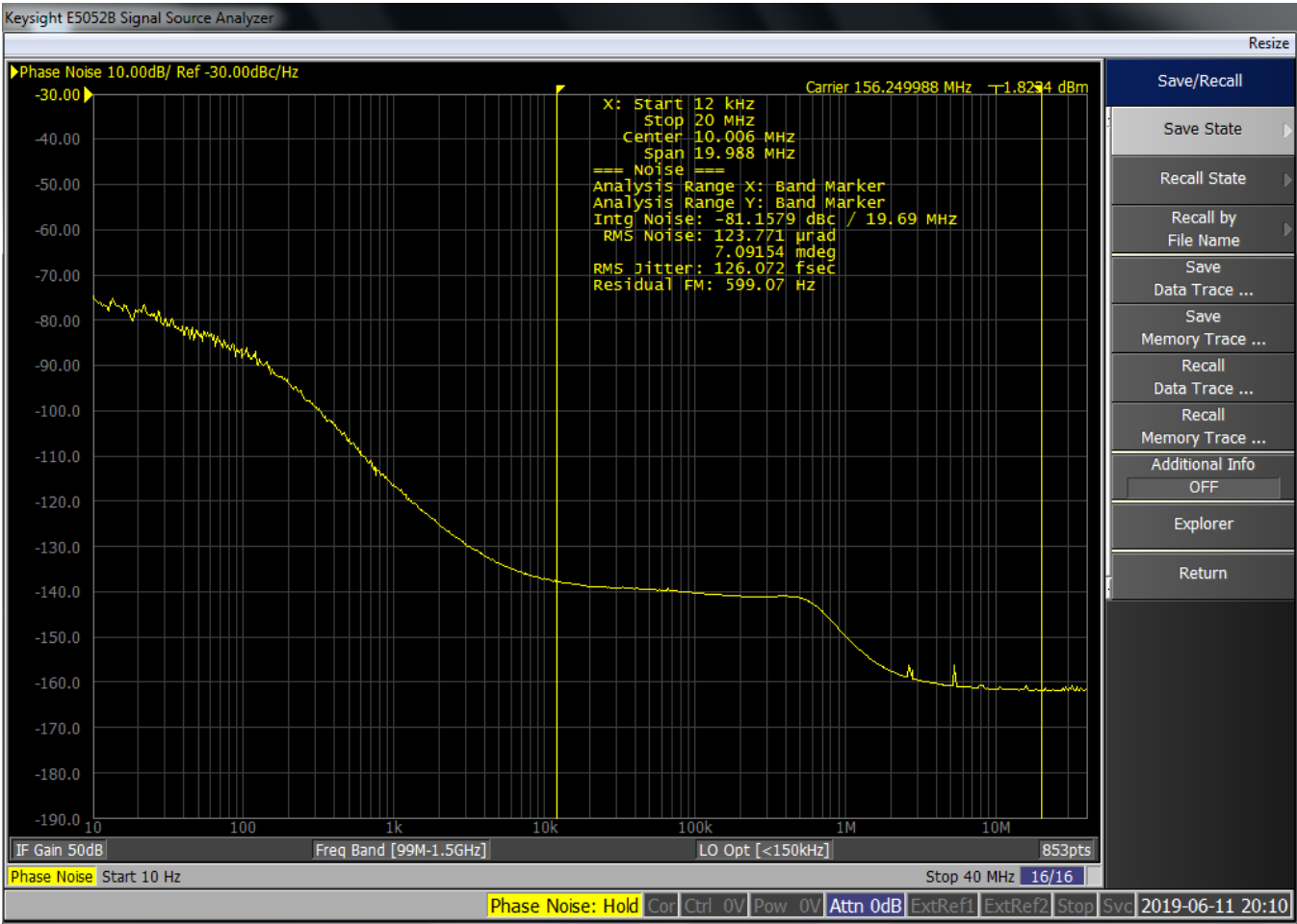
Figure 4. Representative Phase Noise Measurement: F_{OUT} = 156.25 MHz, F_{IN} = 10 MHz, BW = 100 Hz
