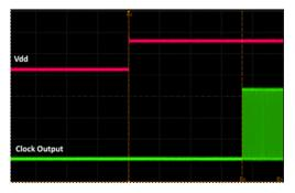
Figure 16. Startup Waveform vs. Vdd
