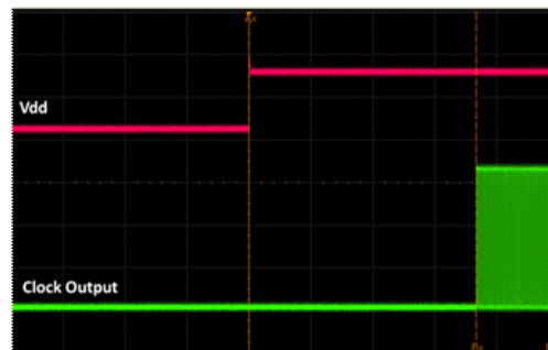
Figure 16. Startup Waveform vs. Vdd
