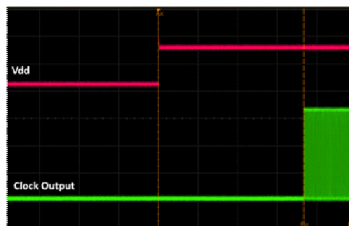
Figure 17. Startup Waveform vs. Vdd
