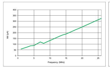
Figure 8. Idd vs Frequency without load
