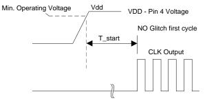
T\_start: Time to valid clock output from power on
