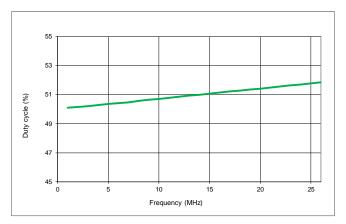
Figure 12. Duty Cycle vs Frequency
