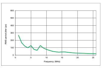
Figure 11. RMS Period Jitter vs Frequency
