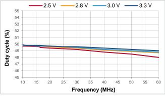
Figure 28. Duty Cycle (Clipped Sinewave)
