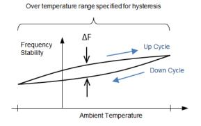
Figure 9. Illustration of hysteresis, where  $\Delta F$  is max frequency difference between up and down cycles across temperature
