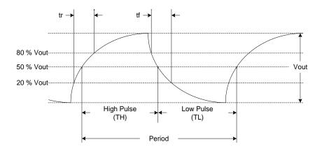
Figure 6. Clipped Sinewave Waveform Diagram<sup>[13]</sup>
