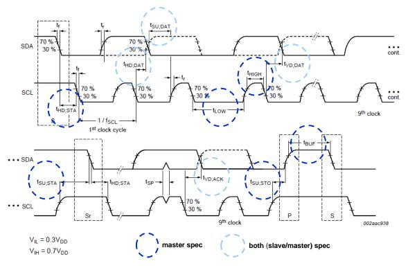
Figure 38. I<sup>2</sup>C Timing Diagram
