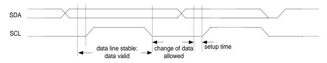
Figure 32. Data and clock timing relation in I<sup>2</sup>C bus
