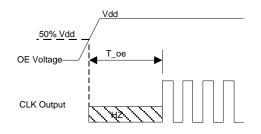
T\_oe: Time to re-enable the clock output
