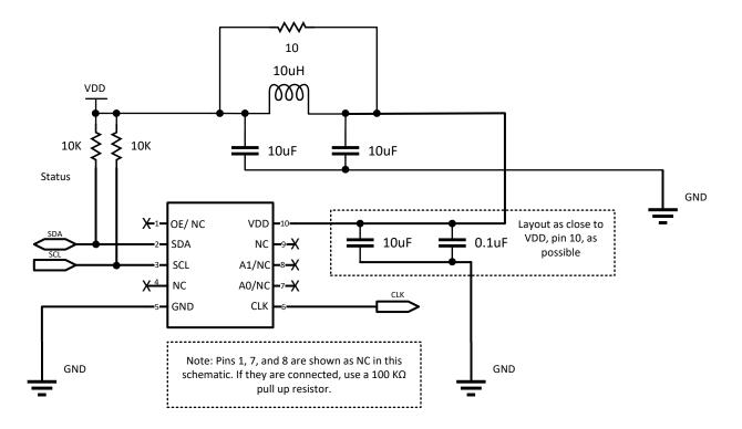
Figure 39. DCTCXO schematic example
