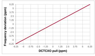
Figure 24. DCTCXO frequency pull characteristic
