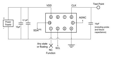
Figure 12. LVCMOS Test Circuit (I<sup>2</sup>C Control), DCTCXO mode for AC and DC Measurements
