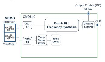
Figure 35. Block Diagram – TCXO
