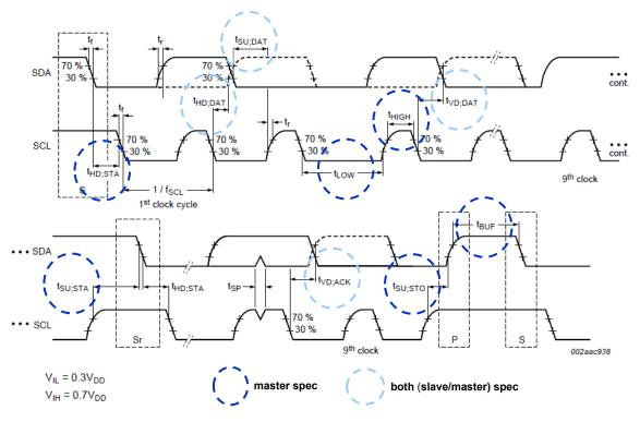
Figure 48. I<sup>2</sup>C Timing Diagram
