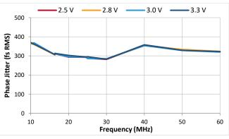
Figure 31. RMS Phase Jitter, DCTCXO, TCXO (Clip Sine)
