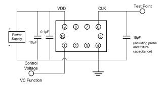
Figure 8. LVCMOS Test Circuit (VC Function)
