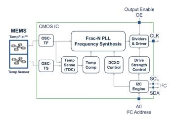
Figure 37. Block Diagram
