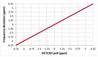
Figure 27. DCTCXO frequency pull characteristic
