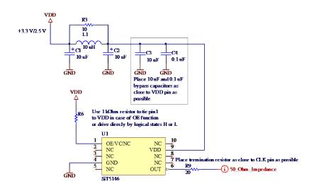
Figure 50. TCXO schematic example
