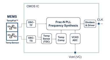
Figure 36. Block Diagram – VCTCXO
