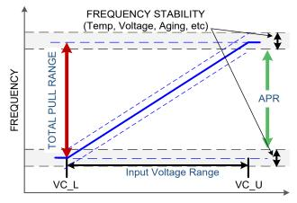
Figure 40. Typical SiTime VCTCXO FV Characteristic
