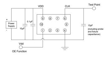
Figure 6. LVCMOS Test Circuit (OE Function)
