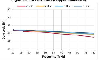
Figure 34. Duty Cycle (Clipped Sinewave)
