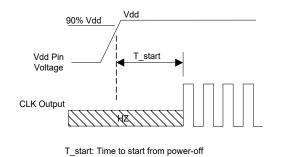
Figure 17. Startup Timing
