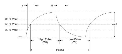
Figure 16. Clipped Sinewave Waveform Diagram<sup>[12]</sup>
