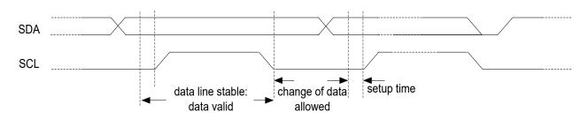
Figure 42. Data and clock timing relation in I<sup>2</sup>C bus
