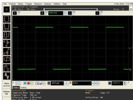
Figure 3. LVCMOS Output Swing ( V_{DD} = 1.8\text{ V} )
