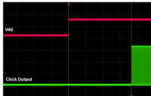
Figure 14. Startup Waveform vs. Vdd
