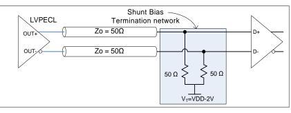
Figure 14. LVPECL with DC-coupled parallel shunt load termination
