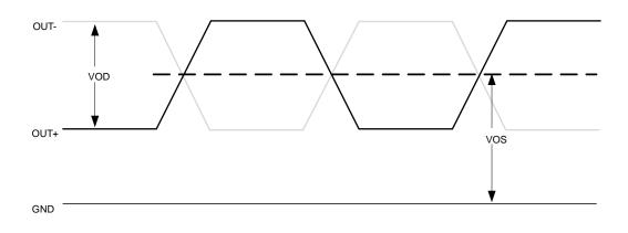
Figure 7. LVDS Voltage Levels per Differential Pin (OUT+, or OUT-)
