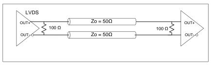
Figure 17. LVDS double DC termination
