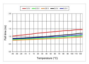
Figure 12. 20%-80% Fall Time vs Temperature
