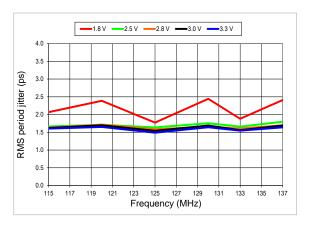
Figure 9. RMS Period Jitter vs Frequency
