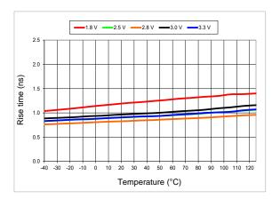
Figure 11. 20%-80% Rise Time vs Temperature
