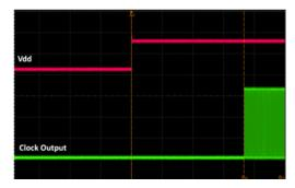
Figure 16. Startup Waveform vs. Vdd
