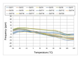
Figure 8. Frequency vs Temperature
