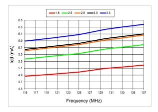
Figure 7. Idd vs Frequency
