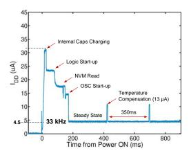
Figure 4. Start-up and Steady-State Current Profile
