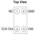
Figure 1. Pin Assignment
