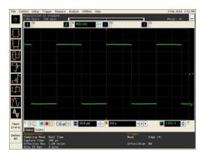
Figure 3. LVCMOS Output Swing  $(V_{DD} = 1.8 \text{ V})$
