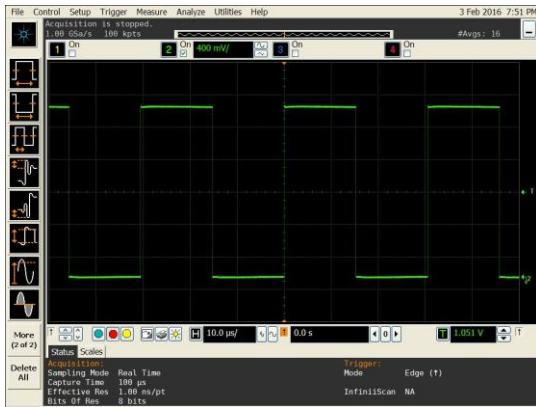
Figure 3. LVC MOS Output Swing ( V_{DD} = 1.8\text{ V} )
