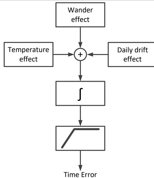
Figure 5: Simulation models of oscillator's time error contributing factors
