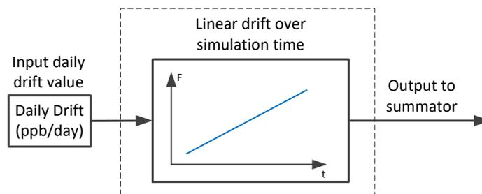
Figure 8: Daily drift (aging) simulation model
