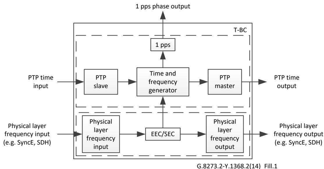
Figure 2: Model of the T-BC defined in G.8273.2
