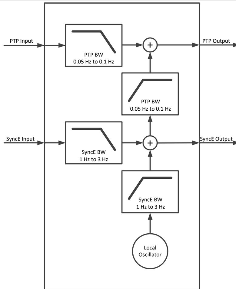
Figure 3: Simulation Model of the T-BC implemented in the software
