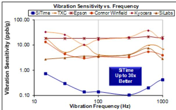
Figure 7: Vibration Robustness [6]
