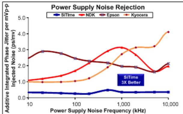
Figure 6: Power Supply Noise Rejection [5]
