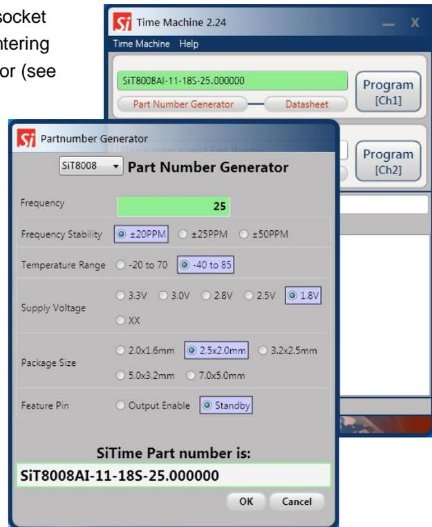
**Figure 2: Time Machine II interface and part number generator enable quick and easy programming of multiple specifications**
