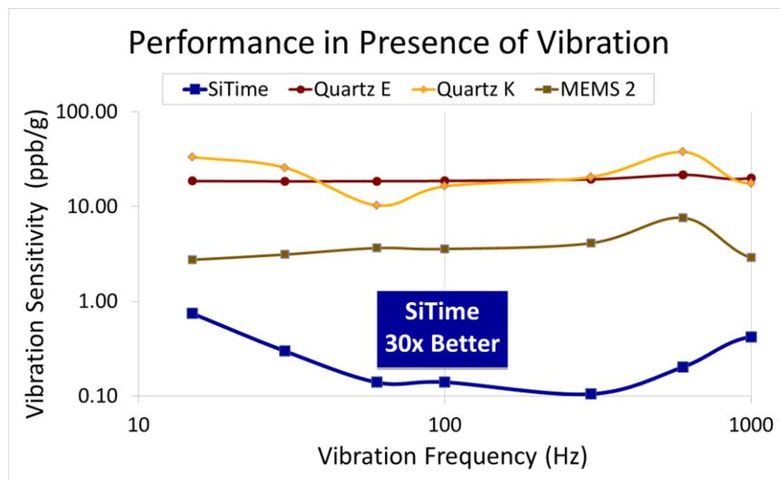
Figure 1: Oscillator sensitivity to sinusoidal vibration
