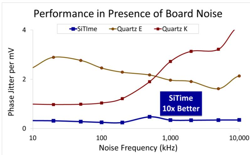
Figure 3: Phase jitter in the presence of 50 mV peak-to-peak power supply noise for SiTime MEMS oscillator (lower line) and quartz oscillators as a function of power supply switching noise frequency
