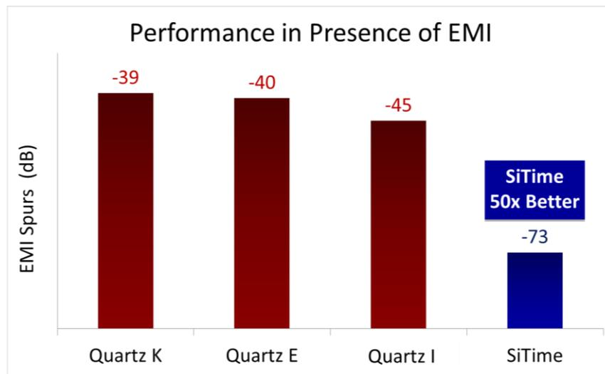
Figure 2: Average EM-induced phase noise spurs on various oscillators
