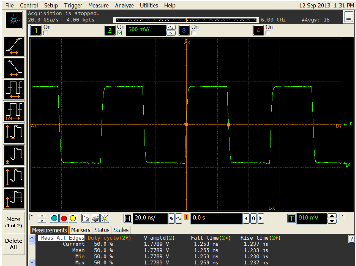
Figure 1. Duty cycle, Rise/Fall time and Amplitude 1.8V
