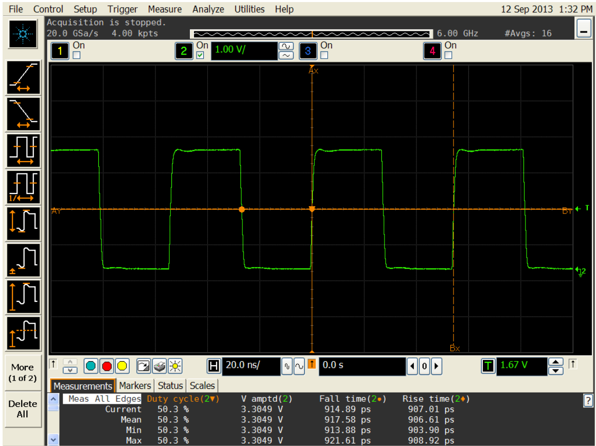
Figure 5. Duty cycle, Rise/Fall time and Amplitude 3.3V
