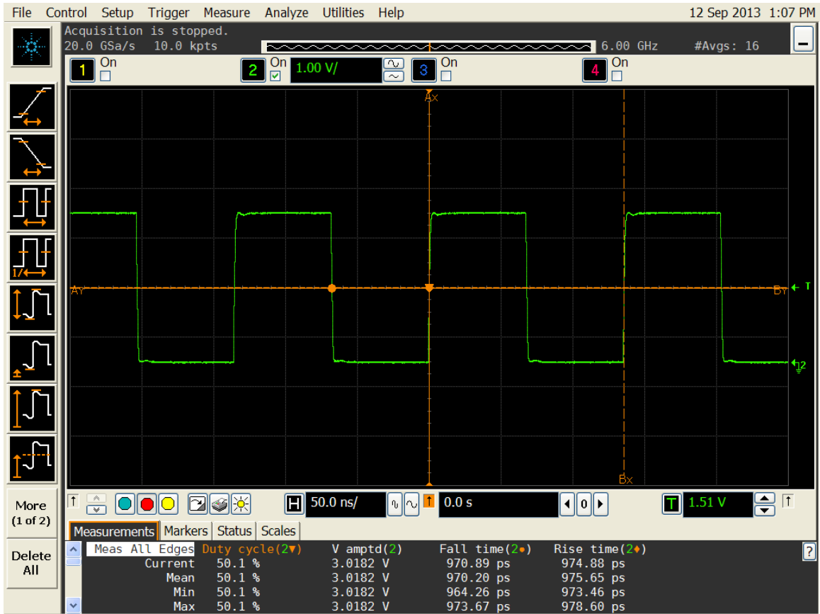
Figure 4. Duty cycle, Rise/Fall time and Amplitude 3.0V
