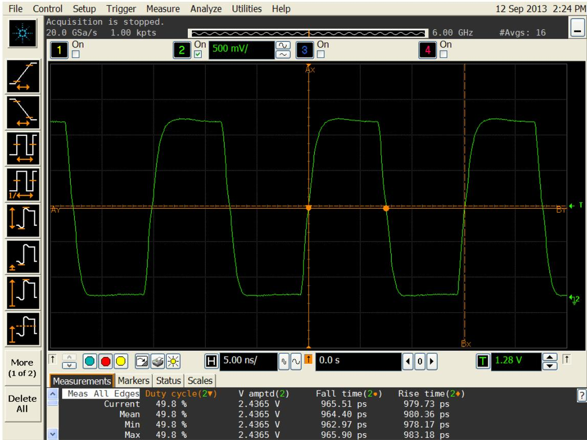
Figure 2. Duty cycle, Rise/Fall time and Amplitude 2.5V
