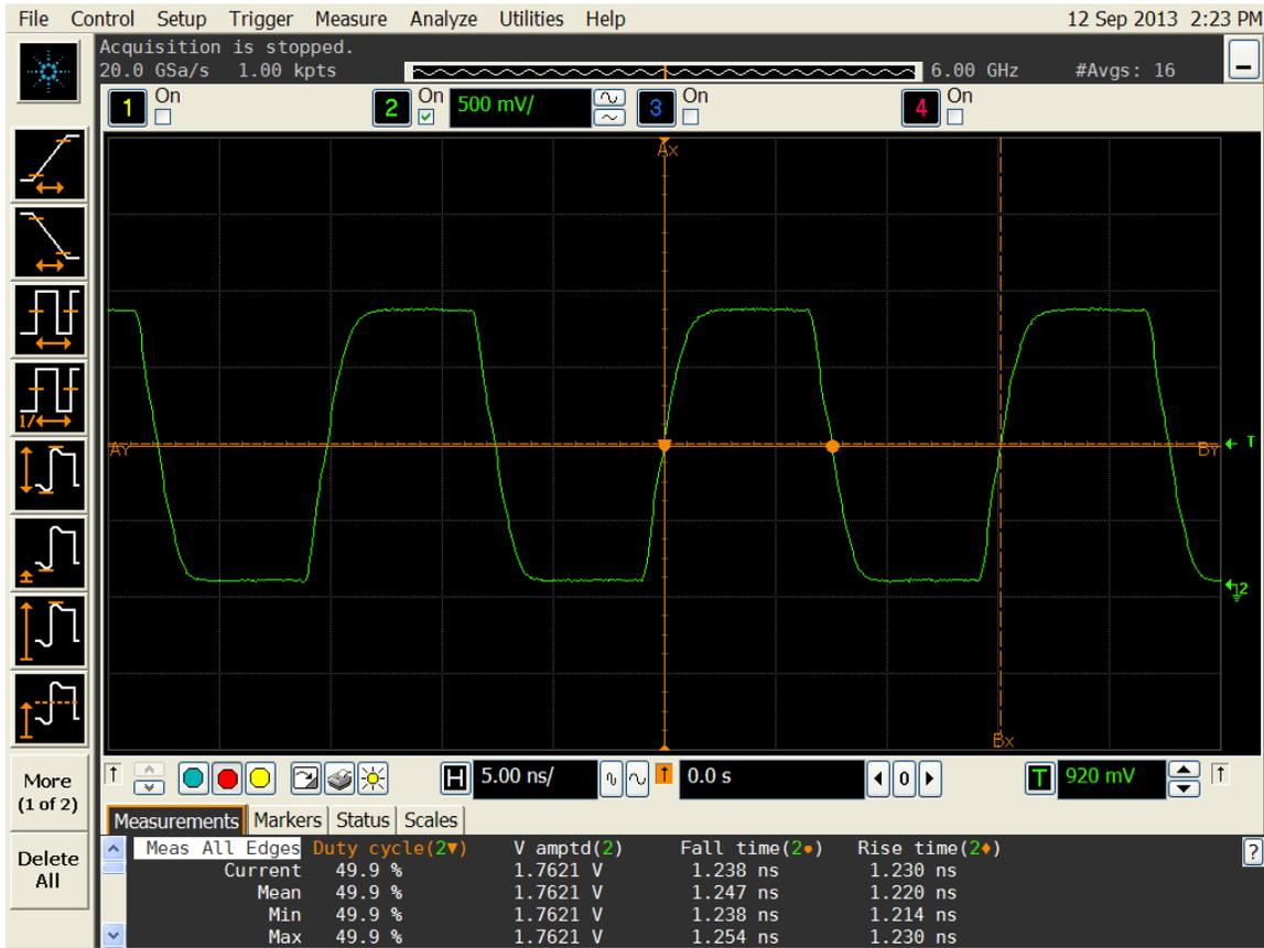
Figure 1. Duty cycle, Rise/Fall time and Amplitude 1.8V
