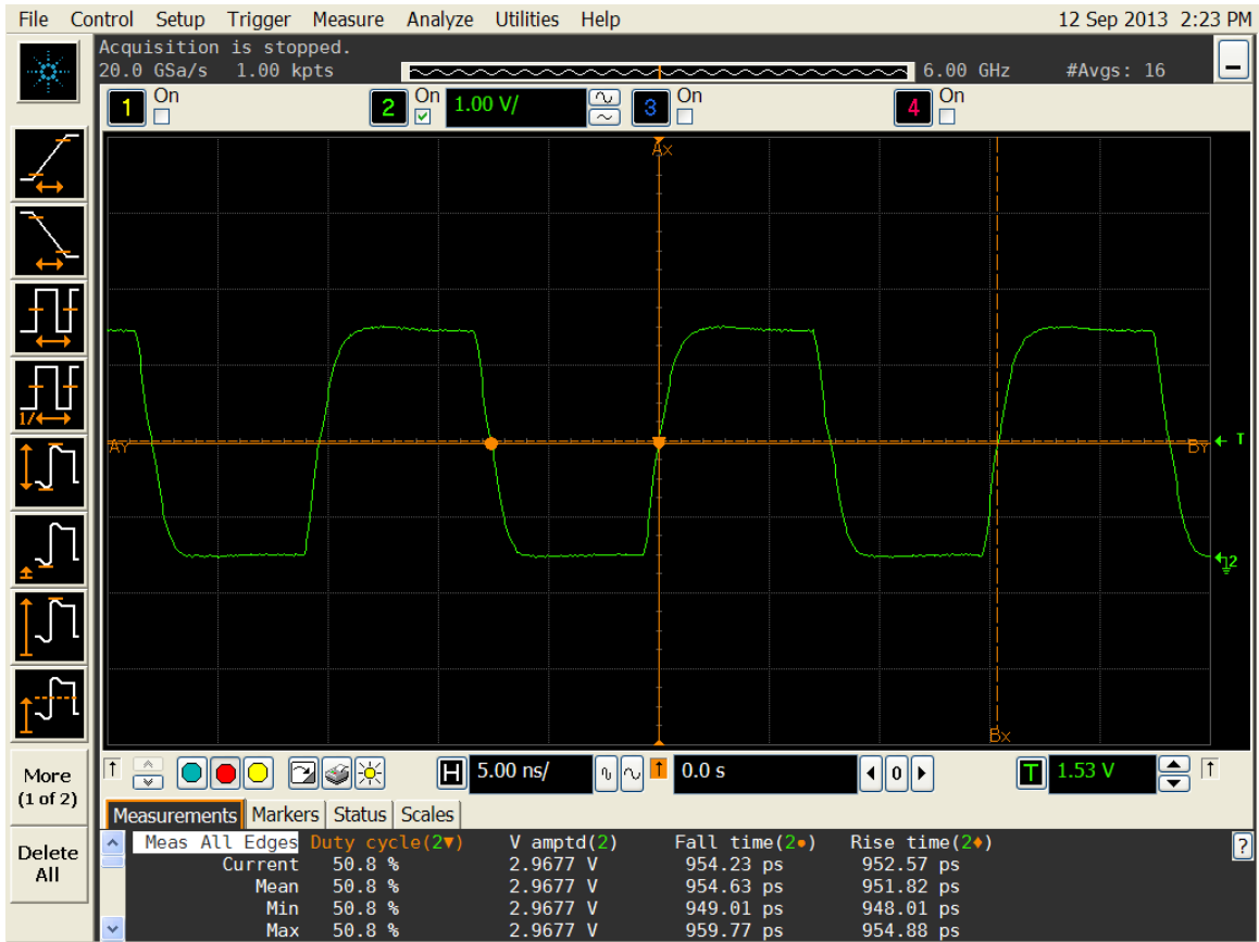
Figure 4. Duty cycle, Rise/Fall time and Amplitude 3.0V
