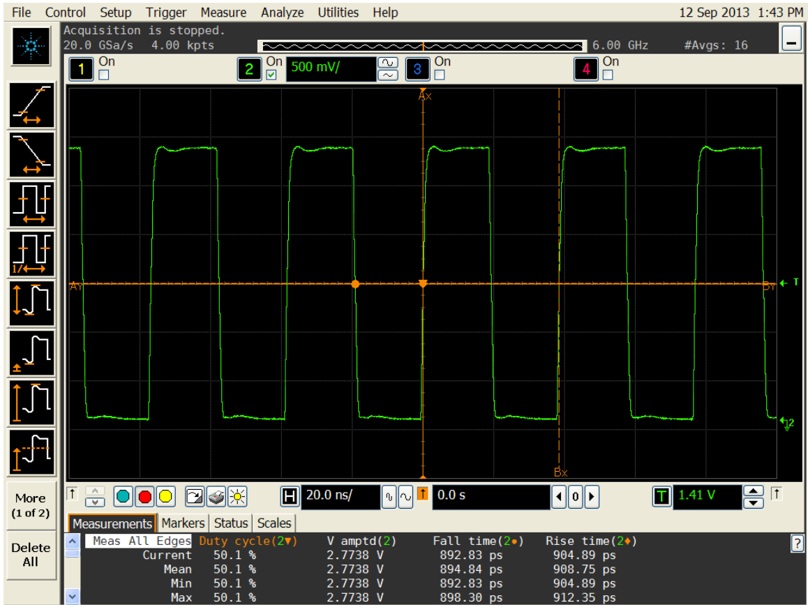
Figure 3. Duty cycle, Rise/Fall time and Amplitude 2.8V
