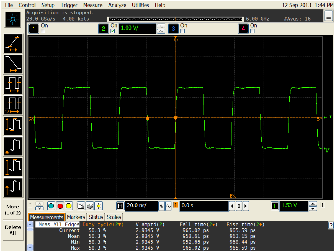
Figure 4. Duty cycle, Rise/Fall time and Amplitude 3.0V
