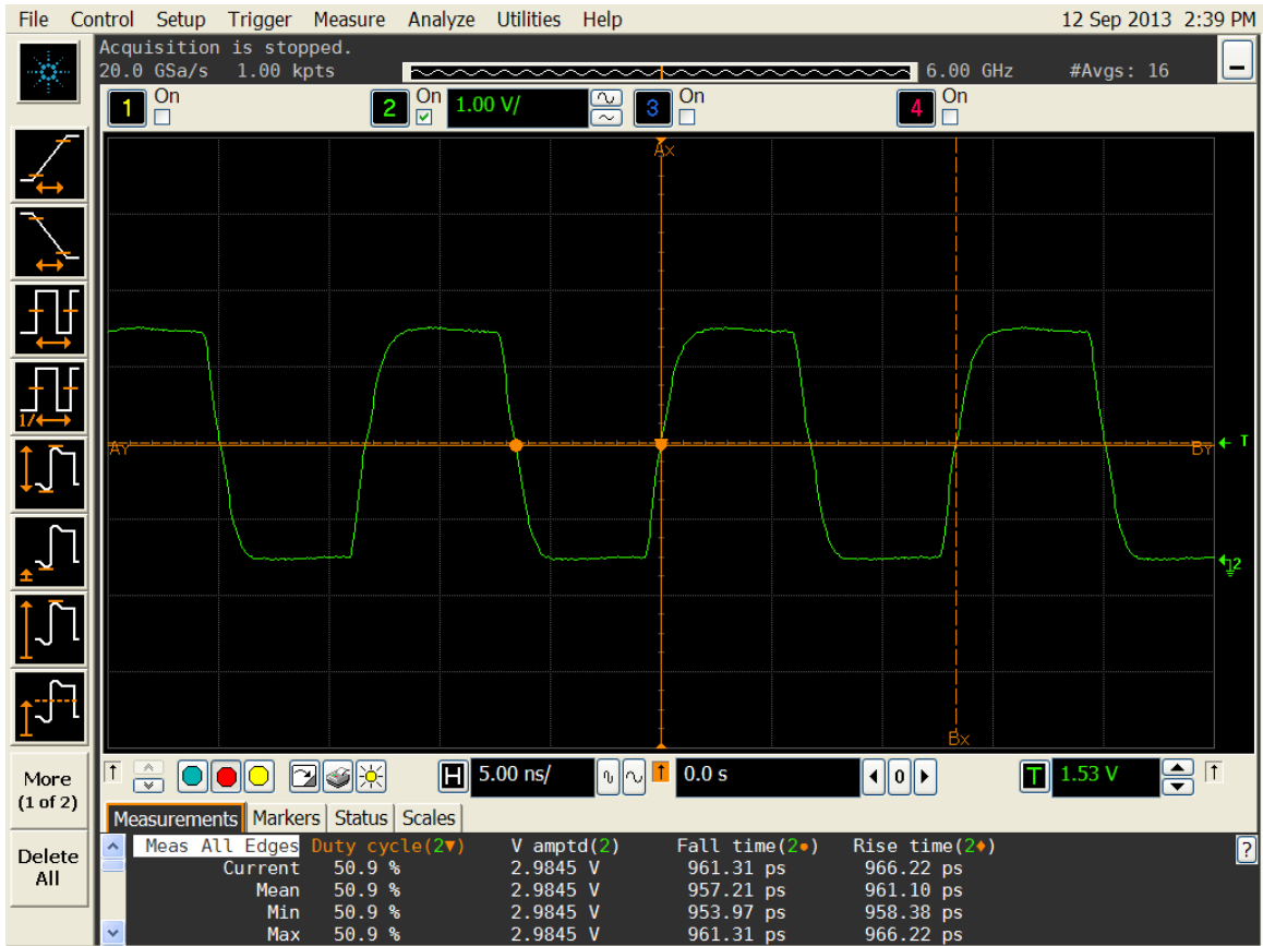
Figure 4. Duty cycle, Rise/Fall time and Amplitude 3.0V
