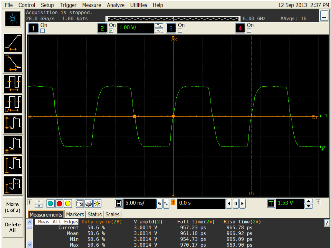
Figure 4. Duty cycle, Rise/Fall time and Amplitude 3.0V
