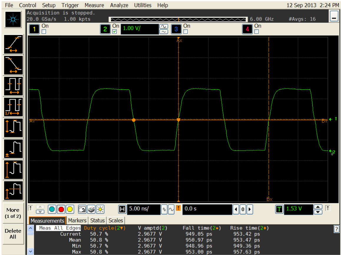
Figure 4. Duty cycle, Rise/Fall time and Amplitude 3.0V
