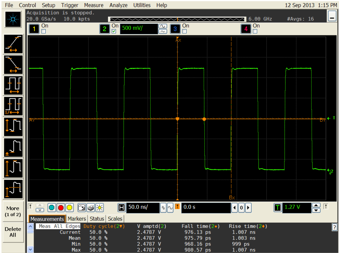
Figure 2. Duty cycle, Rise/Fall time and Amplitude 2.5V
