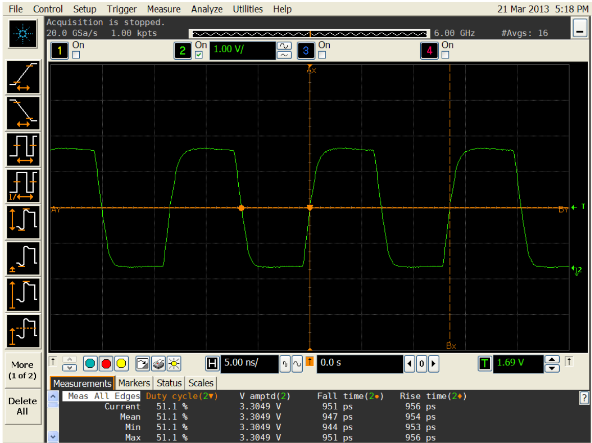
Figure 5. Duty cycle, Rise/Fall time and Amplitude 3.3V
