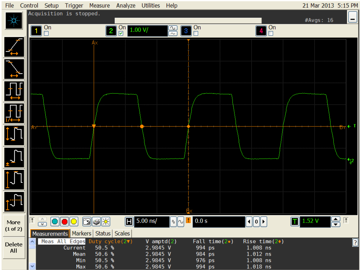
Figure 4. Duty cycle, Rise/Fall time and Amplitude 3.0V
