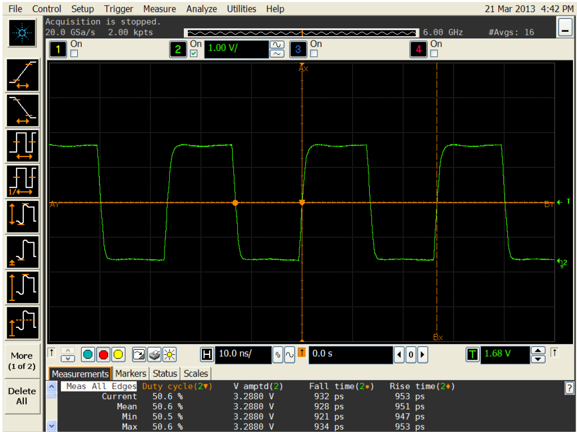
Figure 5. Duty cycle, Rise/Fall time and Amplitude 3.3V
