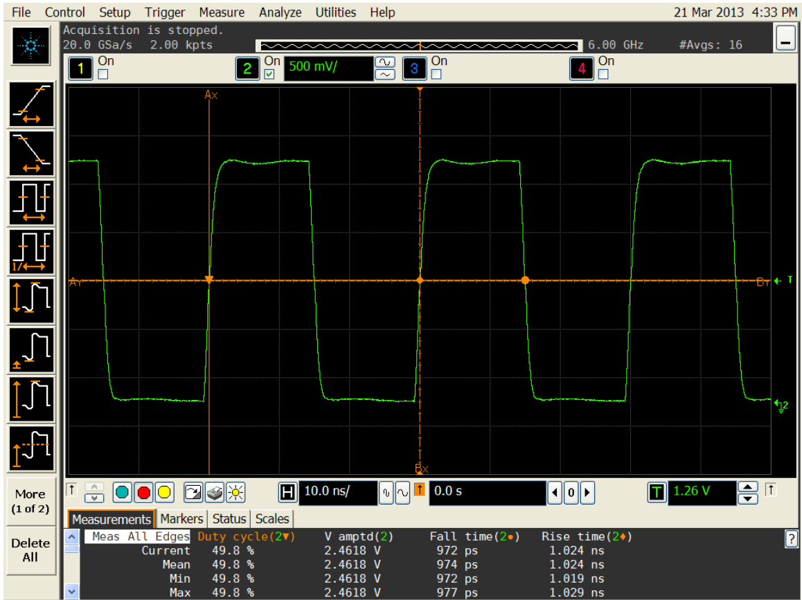
Figure 2. Duty cycle, Rise/Fall time and Amplitude 2.5V
