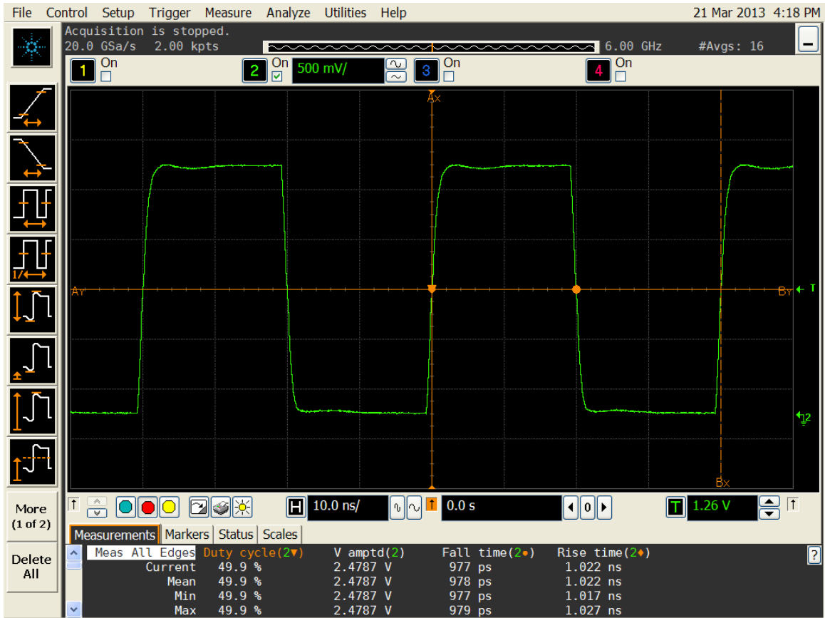
Figure 2. Duty cycle, Rise/Fall time and Amplitude 2.5V
