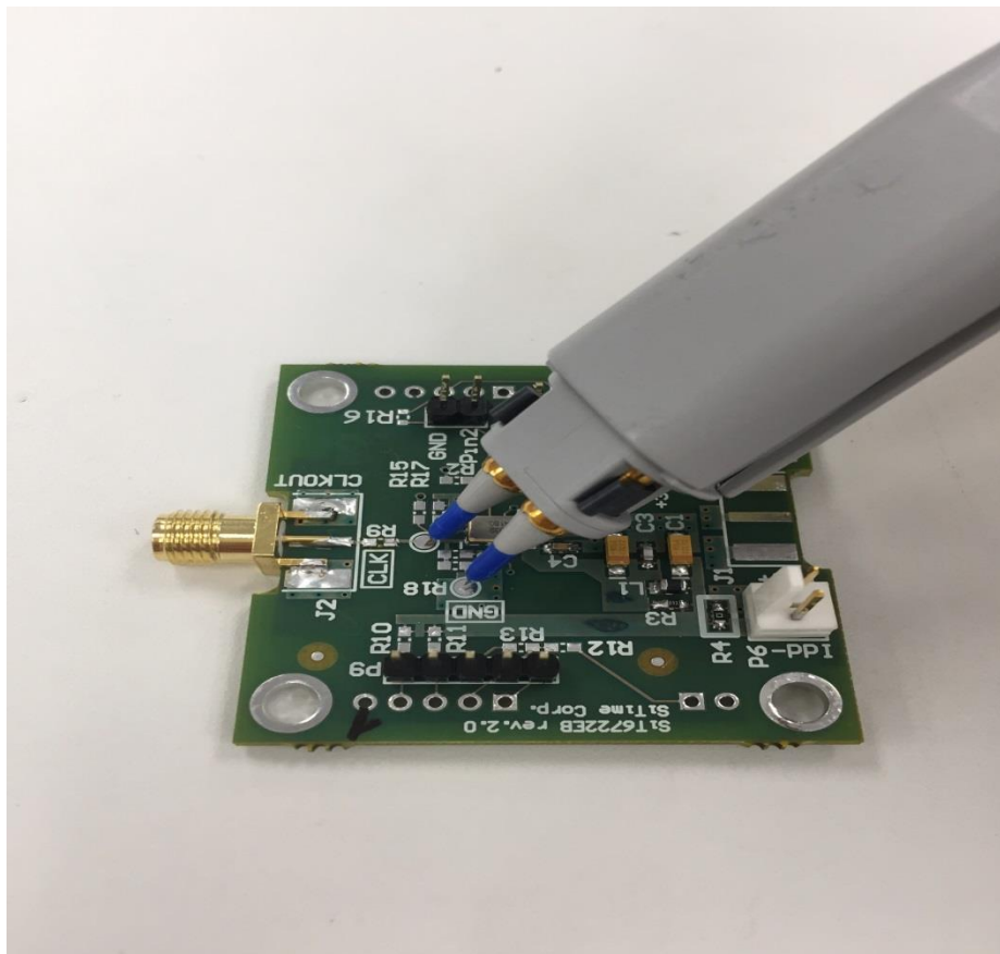
Figure 1: Proper Waveform capturing on SiT6722EB
