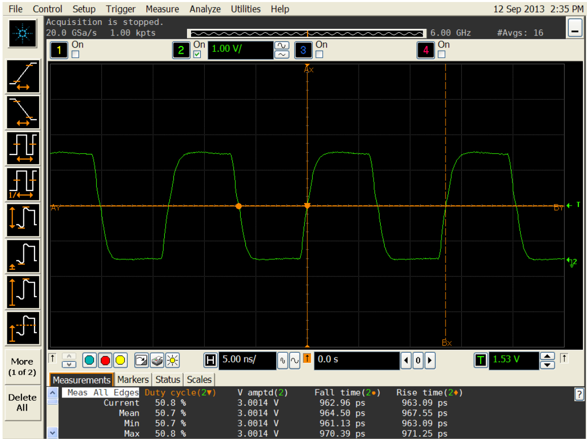
Figure 4. Duty cycle, Rise/Fall time and Amplitude 3.0V
