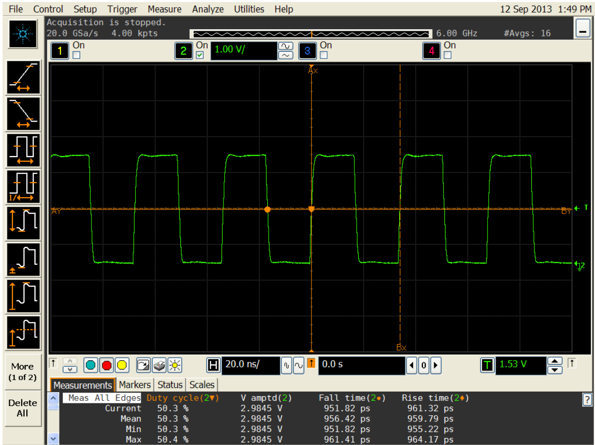
Figure 4. Duty cycle, Rise/Fall time and Amplitude 3.0V
