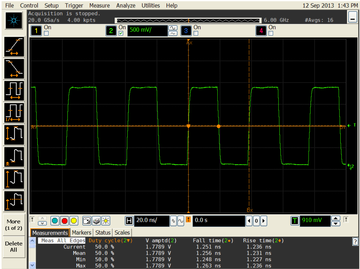
Figure 1. Duty cycle, Rise/Fall time and Amplitude 1.8V
