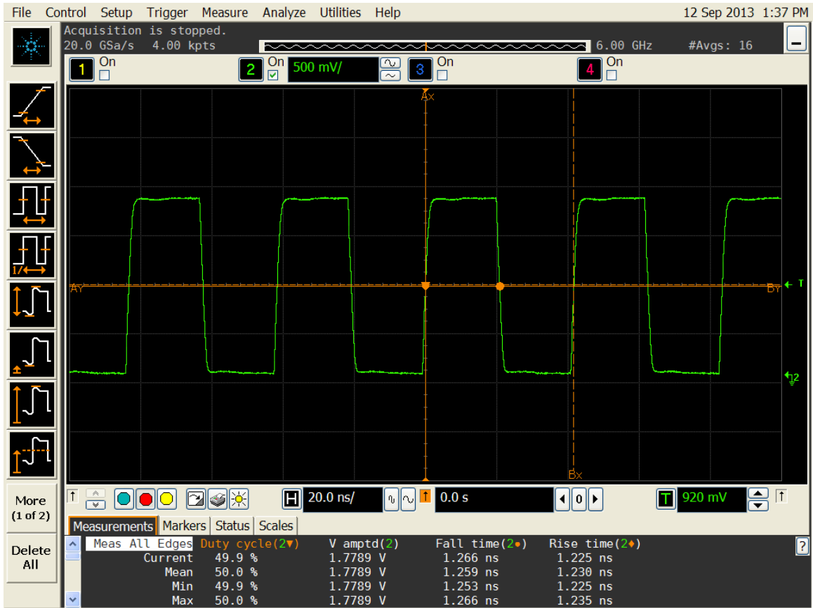
Figure 1. Duty cycle, Rise/Fall time and Amplitude 1.8V
