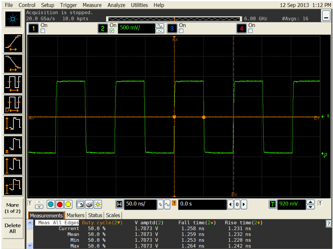
Figure 1. Duty cycle, Rise/Fall time and Amplitude 1.8V
