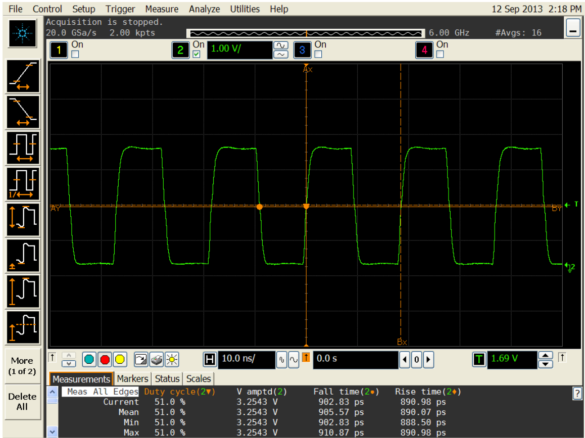
Figure 5. Duty cycle, Rise/Fall time and Amplitude 3.3V
